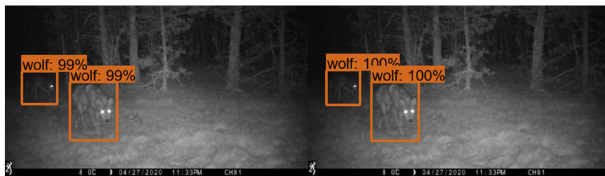
FIGURE 3 Bounding boxes with confidence predictions around a target object. Computer-generated bounding boxes are shown on the left side and human-labeled bounding boxes are shown on the right side.
